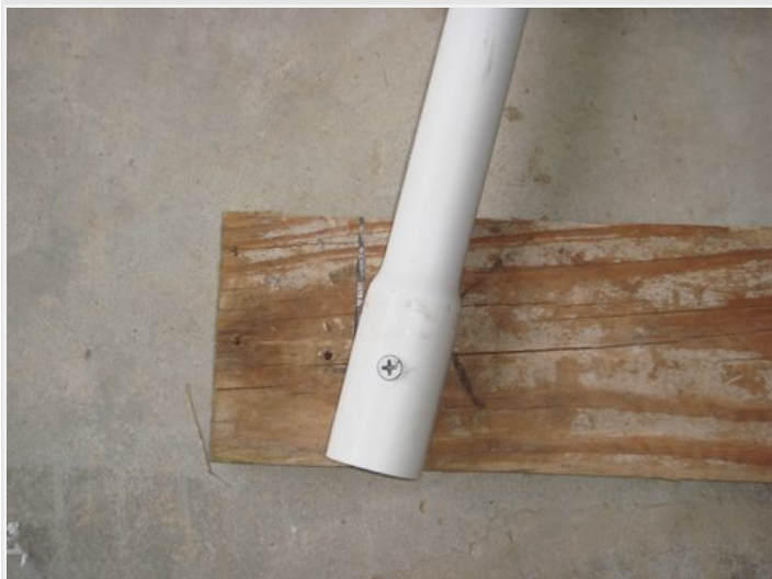
Pre-drill the pipe and use one screw so that the pipe can swivel to whatever angle it naturally aligns to. For now just let the wood "run wild"
